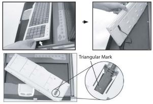
**Please note:** There is a round hole under the drawer, which can be used to pass one finger through allowing for easier removal of the keyboard (pushing upwards).
