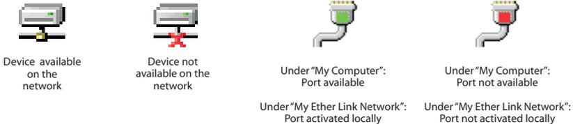
Activated ports appear in Windows' Device Manager under the "Ports (COM & LPT)" branch as "IP-Extender" ports, with their associated COM numbers.
