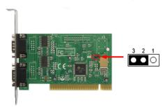
As an option, you can choose to configure the clock frequency of your card by setting the JP15 jumper pins. You can alter this setting by placing the jumper on the pins according to the following chart:
