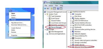
Under the "Universal Serial Bus Controllers" category, new "VIA" host controller devices should now be listed.
