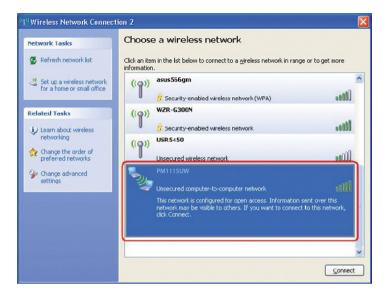
**Note:** If you cannot find the PM1115UW network, then your version of Windows may not be configured to show Ad-Hoc wireless networks. To resolve this issue, you need to use an RJ45 cable to either connect your print server to your network switch or to connect directly to the computer. When the setup is complete, you can disconnect the network cable.
