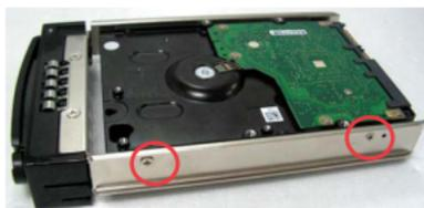
3. Slide the trays back into the enclosure until they are fully seated, then close the arms.
