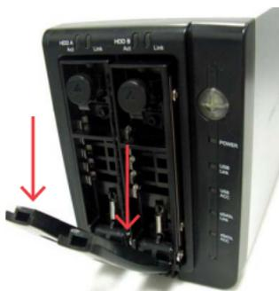
2. Remove the screws holding in the plastic brace from the tray, then secure the hard drive into the trays with the previously removed screws. Repeat for each hard drive tray.
