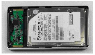
3. Place the foam to fill up the gap between the HDD and enclosure. Assemble the case by sliding on the back cover. No screw is needed.
