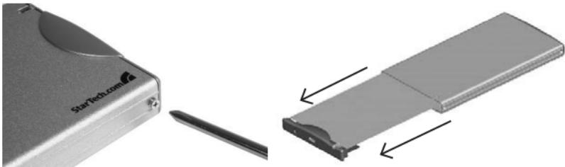
2. Attach the 2.5" SATA hard drive to the connector provided:
