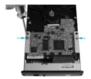
4. Carefully slide the rear panel assembly (with drive attached) into the body of the Enclosure; be cautious that the rear panel assembly is properly aligned with the body of the Enclosure to prevent damage to the LEDs.
