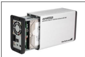
6. Secure the Enclosure tray within the Enclosure, using the screws removed in step 1.
