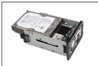
3. Secure the drives to the Enclosure tray, using the provided screws.
