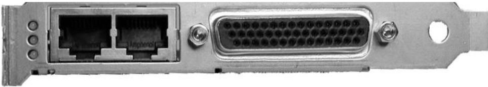
*LEDs WAN LAN Breakout *LEDs are WAN link, LAN link, USB
