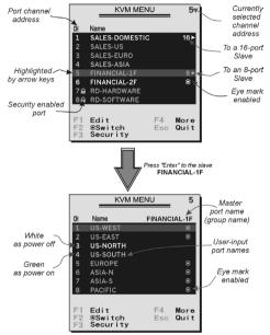
The port number (or channel address) of the currently selected computer is displayed in red in the top right of the screen.
