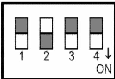
**OFF:** If Pin 2 is in the OFF position, the 110VDSLEXT / GB / EU will operate in Interleave mode, with communication protection for up to 250ms of impulse noise with latency less than 6 ms
