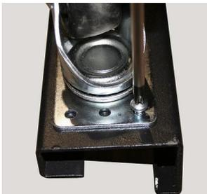
4. Attach the casters, which are included with the packaging, to the legs of the 2POSTRACK. Use a Phillips screwdriver and screws to mount the casters to the legs of the unit.
