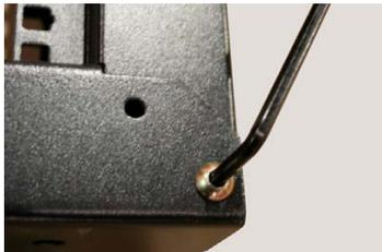
2. When the panels are aligned, the holes should match up with each other allowing you to use the Allen Key to fasten each corner with the nuts and bolts provided.
