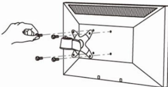
**WARNING!** Do not over-tighten the screws and stop immediately if you encounter resistance to avoid damage to your display. Ensure that all spacers and screws being used are the same length and thread type.
