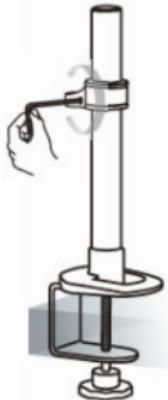
2. Slide the Monitor Mount (2) onto the Support Post (1) until it rests on the Collar (7) and tighten the set screw using the M3 Allen Wrench (15).
