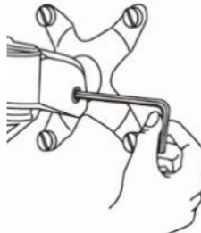
To increase / decrease swivel resistance, adjust the set screw located on the side of the Monitor Mount bracket at the Support Post, using the M3 Allen Wrench (15).
