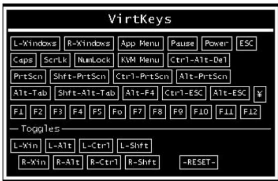
Clicking any button in the top half of the window simulates pressing and releasing the indicated key. In the bottom area of the screen, clicking will simulate the indicated Meta key being pressed. You may then click in the top part to send another key and release the Meta key at the same time. Alternatively, you may move the mouse outside this window, press the regular key, and then choose **-RESET-** to release all depressed keys.
