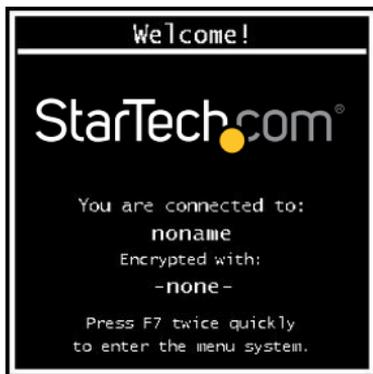
One of the unique features of this product is the VNC menu system. Whenever you see a window with a dark blue background and grey edges, this window has been inserted into the VNC data stream so that it is effectively laid over the existing video. These menus allow you to control the many features of the CABCONS1716I without using the web interface or a custom client.
