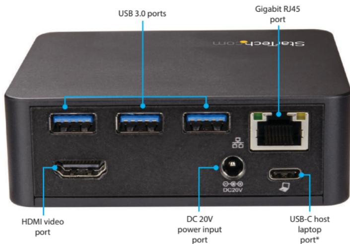
\*USB-C host laptop port connects to your computer only (supports connection of laptop to computer for data, DP Alt Mode and USB Power Delivery.)
