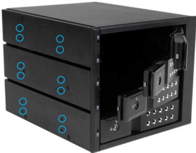
3. Hold the HSB4SATSASBA into place by lining up the screw holes on HSB4SATSASBA with the corresponding mounting holes in your 5.25in bays. Next, fix the HSB4SATSASBA to your 5.25in bays by screwing 4 of the included screws into any of the installation holes on both side of the 5.25" bay (8 screws in total).
