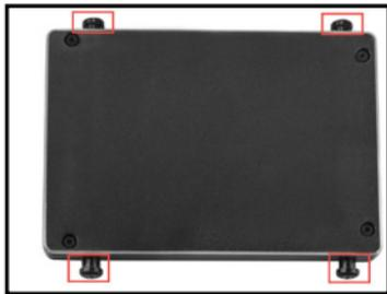
*Installing the four drive screws into the hard drive*
