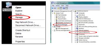
Double-click on the "Ports (COM & LPT)" option. The appropriate number of additional COM ports should be visible. The port(s) are ready to connect to new devices.
