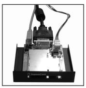
Remove the cover from a 3.5" drive bay, on the front panel of the host computer case, then feed the remaining ends of the cables used in step #1 through the open bay:
