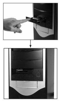
4. Once the ExpressCard Bay has been inserted into the computer case, fasten it to the computer chassis, as you normally would a 3.5" drive (i.e. CD-ROM Drive, etc.), and connect the remaining ends of the cables (see steps #1 and #2) to the appropriate ports as outlined on the following page:
