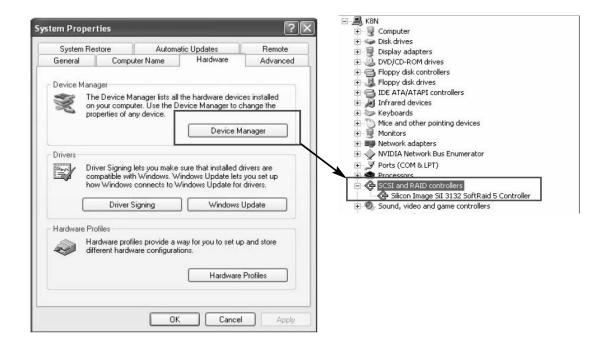
2. To view information about the devices attached to the controller, right click the **Silicon Image Sil 3132 Serial ATA Controller** and select Properties from the context menu, then select the tab labeled **Device Info**.
