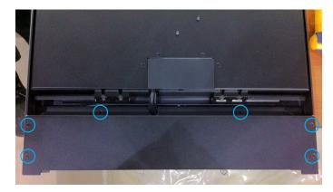
3. Unscrew the nut indicated with a wrench or socket(8mm).
