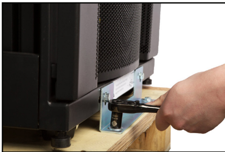
Removing the Bolts
