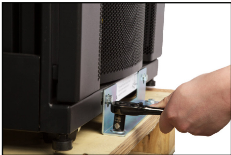
Removing the Bolts
