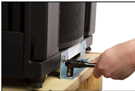
Removing the Bolts
