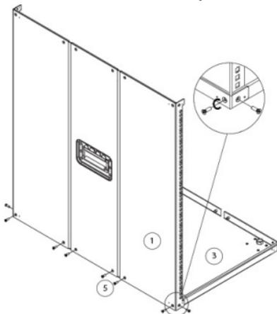
3. Line up the plastic corner caps (#4) with the holes on the corners of the panels. Use the M3 (8 mm) flat-head Phillips screws (#6) to attach the corner caps (#4) to each of the eight corners on the rack.
