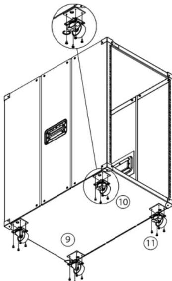
**Warning!** To prevent bodily injury, please make sure that the rack is installed in a structurally sound environment with a level floor, and that all of the hardware has been assembled securely and checked for stability before loading equipment. When installing equipment into the rack, start from the bottom of the rack first and move upwards, keeping the heaviest equipment at the bottom to avoid a situation where the rack becomes top heavy.
