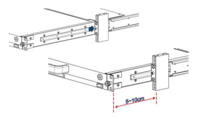
5. Install one of the Blockers onto the back of the console as shown, and use the included screw to secure it. Repeat on the other side.
