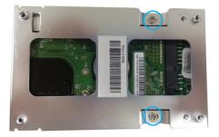
6. Reassemble the enclosure by slide the HDD tray with connected hard drive back into the enclosure.
