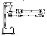
4. Connect the power adapter from an available AC outlet to then enclosure. Turn on the unit by Pushing the Power button at the back of the unit.
