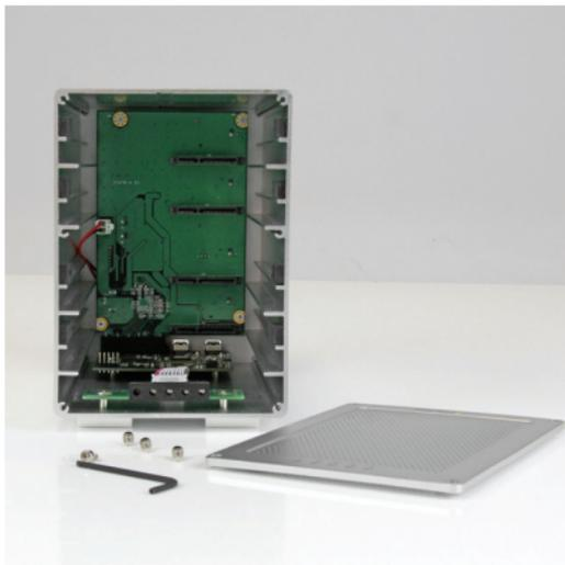
3. On each of your four 3.5in hard drives, place HDD mounting brackets from each of your HDD mounting kits on either side of the drives, aligning the pegs with the hard drive mounting holes. Then with your hard drive labels facing upward, slide each of your four 3.5in hard drives into an available drive bay with the SATA connector facing inward, using the HDD bracket to align the slot.
