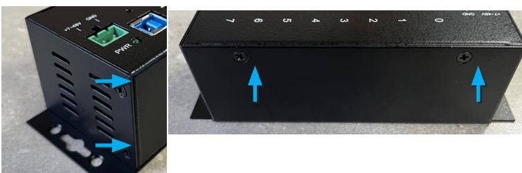
2. Carefully remove the top metal panel from the USB Hub, and remove the four screws, located on the upper PCB, using a Philips-head screwdriver.
