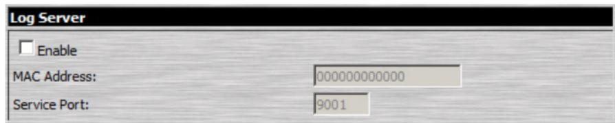
The screenshot shows a configuration window titled "Log Server". It contains three main elements: a checkbox labeled "Enable" which is currently unchecked; a text field labeled "MAC Address:" containing the value "000000000000"; and a text field labeled "Service Port:" containing the value "9001".
