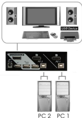
1. Plug a monitor into the Console DisplayPort connector; plug a USB keyboard and a USB mouse into the dedicated USB keyboard and mouse ports on the KVM switch.
