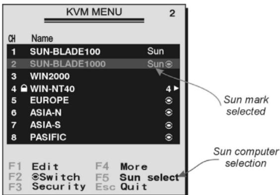
**NOTE:** It is unnecessary to switch the Sun mark ON or OFF if an authentic Sun keyboard is being used on the console. In other words, you must ensure that the Sun-marked port has not been selected if you are already using a Sun keyboard. With different types of keyboard and computer, the Sun Mark must be set up in compliance with the following instruction:
