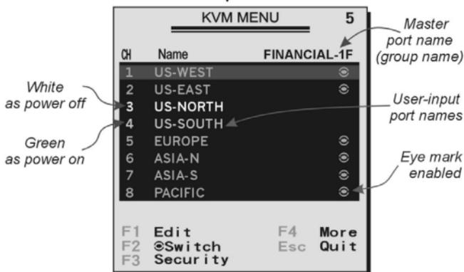
By hitting the left <CTRL> key twice within two seconds, you may see the 'Hotkey Menu' if it is enabled (an OSD option). Or, by hitting the left <CTRL> key three times within two seconds, you will see a 'KVM MENU' screen showing a list of the computers with corresponding channel addresses, names and status.
