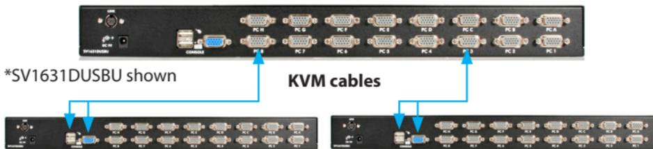
The maximum number of computers controlled by a Master/Slave configuration with all 8-port KVM switches used is 64, with 8 Slaves and each Slave connecting to 8 computers:
