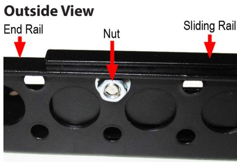
**NOTE:** If possible, do not have the screws go through all 3 Rails, as this will prevent the rails from sliding. If possible, try to only have the screws go through the Sliding Rail and one End Rail.
