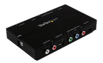
**NOTE:** This Device can capture at 1080p at 30/50/60 frames per second. Live Video output will always display at 30 frames per second.
