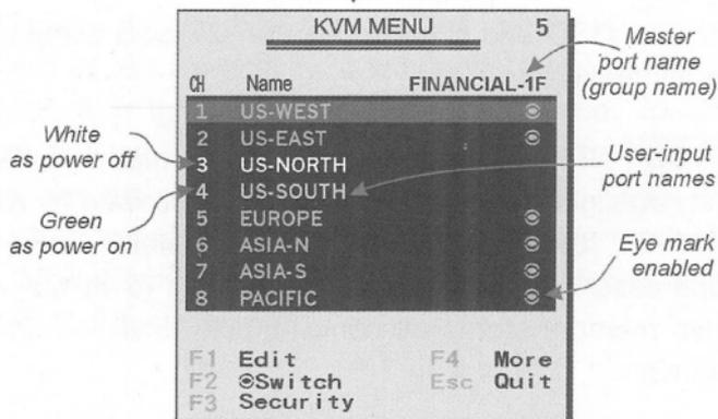
The port number (or channel address) of the currently selected computer is displayed in red in the top right of the screen.
