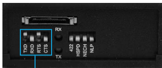
Terminator Enable/ Disable Switches
