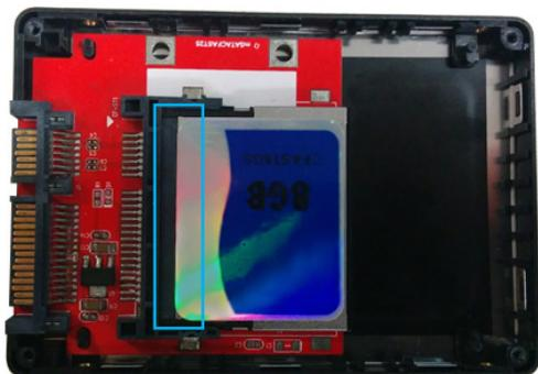
**Note:** The connector on your CFAST card is keyed so the card will only fit one way.
