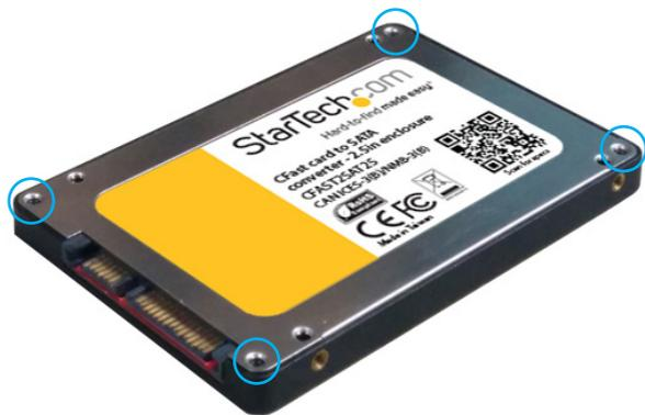
2. With the label facing upward connect your CFAST card to the CFAST receptical connector on the adapter.
