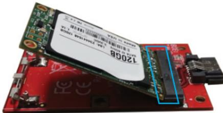
2. Gently apply pressure to the top center of the drive until it locks into place on either side of the SSD clip. To release the drive from the SSD clip, pull up on the top of the clip using the levers attached to either side of clip.
