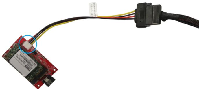
4. Plug the SATA port on the SAT32MSATM with installed drive into an available SATA port on the system motherboard.
