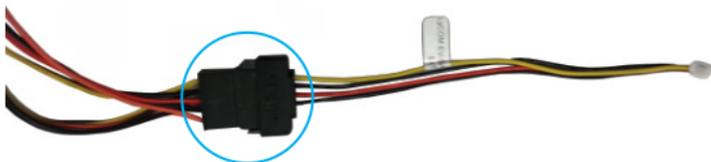
3. Connect the 4-Pin portion of the included SATA Power to 4-pin Power Adapter to the 4-pin power connector on the SAT32MSATM.
