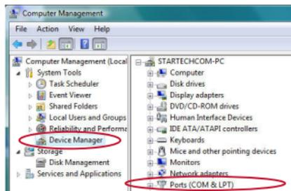
Double-click on the “Ports (COM & LPT)” option. The appropriate number of additional COM ports should be visible. The port(s) are ready to connect to new devices.
