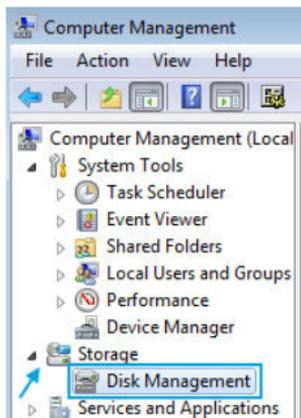
3. A dialog window should automatically appear, asking you to initialize the drive. Depending on the version of Windows, it will give you the option of either creating an "MBR" or "GPT" disk. GPT (GUID partition) is not compatible with some older operating systems, while MBR is supported by newer and older operating systems.
