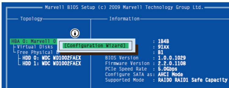
4. Use the arrow keys to scroll through the list of free physical disks to select the drives that will be part of the RAID set. Press Space to select/de-select a disk.
