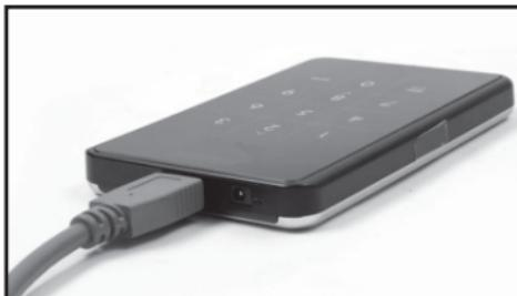
**OPTIONAL:** If the USB port does not provide enough power to the drive/enclosure, use the provided USB to DC adapter cable to connect the DC port on the enclosure to an additional USB port on the host computer.
