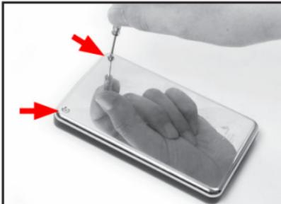
2. Using the small groove located along the top edge of the enclosure, remove the back panel to expose the interior drive bay.
