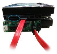
Using the remaining included SATA Cable, connect the SATA Host Interface connector on the S322SAT3R to an available SATA Interface on your Computer System.
