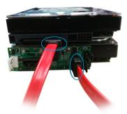
4. Connect an available **SATA Power Source** in your **Computer System** to the SATA (Power) connector on the second **HDD/SSD**.
