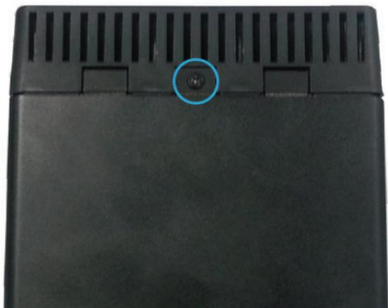
2. Slide the "front panel" upward toward the top of the enclosure.
