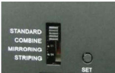
3. Toggle the rear power switch to the on position then press and hold the "Set RAID button" as you power on the enclosure by pressing the "Front Power Button".
