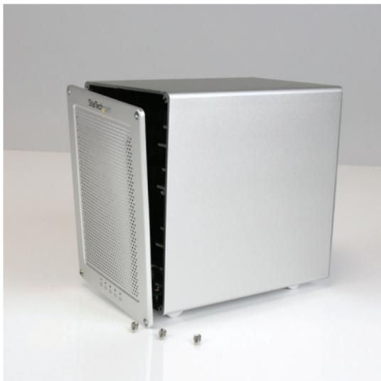
5. Using the included Allen key, drive each of the four screws back into the enclosure through the front place plate.
