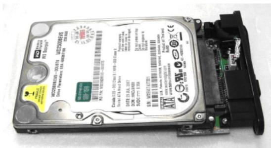
3. From the bottom attach 2 screws to secure the hard drive to the rear panel.
