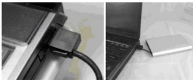
**NOTE:** A DC power connector for an external power adapter is located under the built-in USB cable. This would be necessary for any hard drives that cannot draw enough power from the USB port alone.
