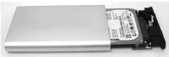
5. Attach two screws. You can now attach the enclosure to a computer system via the integrated USB cable.
