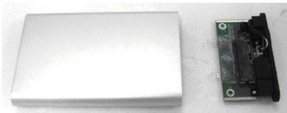
2. Attach the hard drive to the rear panel by simply sliding the hard drive on the 7+15 SATA connector on the rear panel.
