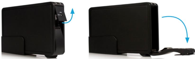
3. Place the hard drive into the SAT3510BU2E, SAT3510BUEGB, SAT3510BUEEU. The printed label on the hard drive should be on the right hand side, with the SATA connector on the lower half of the drive.
