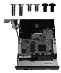
4. Fasten the front panel (with drive attached) to the body of the Enclosure; be cautious that the drive and front panel are properly aligned with the body of the Enclosure, to prevent damage to the LEDs.
